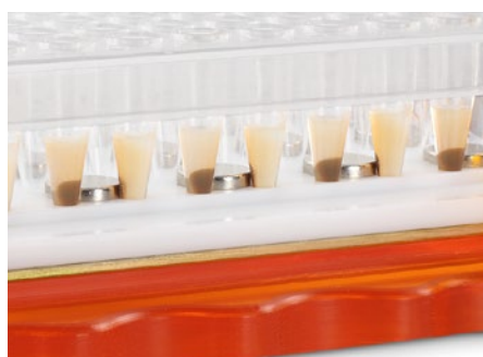
Figure 2. Separation of magnetic beads in microplate format
