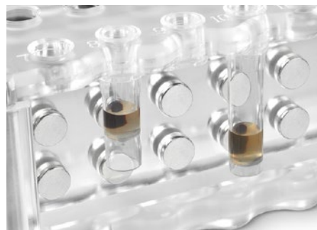
Figure 4. Separation of magnetic beads in tube format
