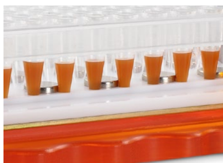
Figure 2. Separation of magnetic beads in microplate format
