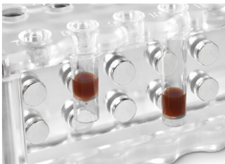
Figure 4. Separation of magnetic beads in tube format
