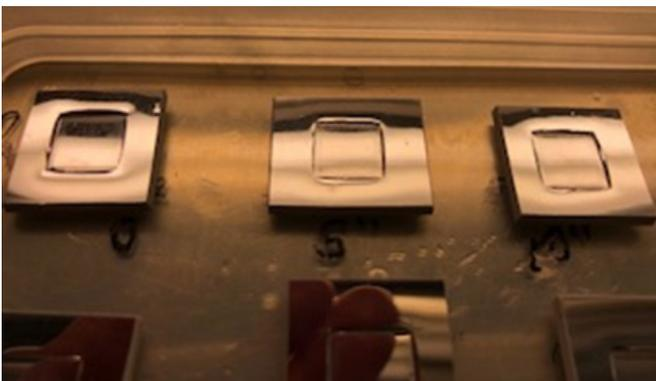
For the dosage experiments the samples were placed under prewarmed germicidal recirculator (UVR-M) for 0, 5 and 10 seconds at distance of 11 mm from the lamp. The UVC dosage is calculated to be 0, 55 and 110 mJ/cm<sup>2</sup>
