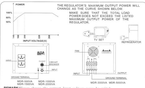
**REMARK:**Please choose the correct Input voltage range by switch the switch lock on the rear panel before you turn on this regulator. Any wrong selection of the Input voltage range may cause the damage of the Regulator.
