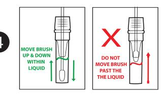
Hold vial steady and move brush up and down rapidly inside the tube 10-15 times without moving the brush out of the liquid.
