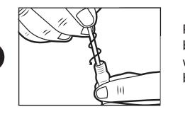
Pick up vial and hold steady in one hand. Slowly twist brush into iSWAB vial with a corkscrew motion. There will be resistance, but push brush all the way to the bottom of tube.
