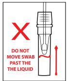
Hold vial steady and move swab up and down rapidly inside the tube 10-15 times without moving the swab out of the liquid.
