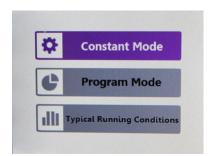
1. Use the up and down arrow keys to select constant mode, then press the enter key to move to the next page.
