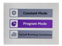
1. Use the up and down arrow keys to select program mode, then press the enter key to move to the next page.
