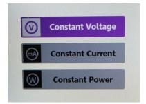
2. Use the up and down arrows to select which parameter should be kept constant. Press the enter key to move to the next page.
