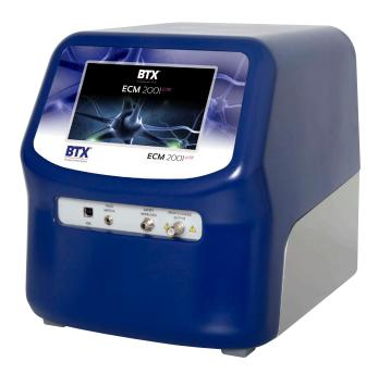
The ECM 2001 LITE is a multifunctional electrofusion and square wave electroporation generator. The ability to generate both AC and DC waves enables fast and efficient cell fusion for hybrid cell formation and nuclear transfer applications. This system is powerful enough to yield high transfection efficiencies for cell lines and difficult to transfect cell types including stem cells and primary cells. The gentle square wave pulse also allows for high cell viability of these cell types.
