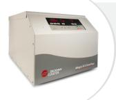
The Allegra X-5 clinical air-cooled benchtop centrifuge is designed specifically for the clinical laboratory which offers high throughput for 13mm and 16mm blood tubes and additional adapters that are compatible with Beckman Coulter Diagnostic instruments (DxC, DxI, AutoMate).
