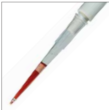
Liquid passes through conventional filter pipet tips causing cross-contamination.
