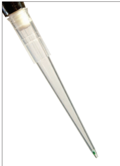
Axygen Maxymum Recovery tip after dispensing 100 µL sample
