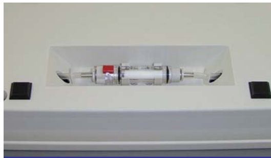
Air Filter Unit
