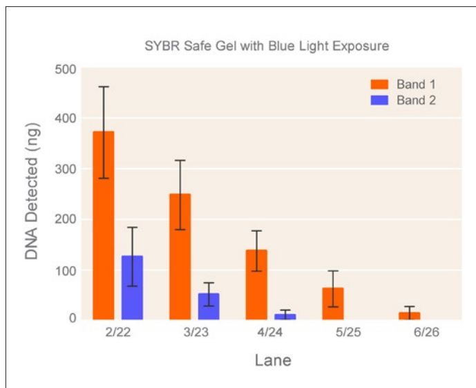
Figure 2. DNA quantification detection limit. The amount of total DNA detected, as determined from calibrating samples to the Axygen 1 Kb DNA ladder, decreased across the gel in direct relationship to the decreasing amount of DNA loaded. Representative data from a SYBR Safe stained-gel illuminated with blue light is shown. Band 1 ~6107 bp, Band 2 ~1746 bp.
