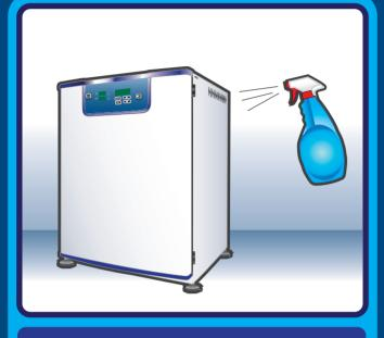
CO2 Incubator needs to be cleaned with a disinfectant or detergent first and then rinsed with sterile water followed by 70% alcohol.
