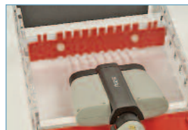
reversible loading guides sit directly above each well to provide a convenient loading template for single- and multi-channel pipettes
