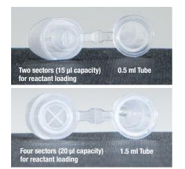
Vertical tab eases handling of tubes in rotors, racks, heat blocks and baths. Hazardous aerosols are vented out the back of the tube and away from the researcher by pressing the levered TabTop. 0.5 ml tubes feature two sectors (15  $\mu$ l capacity) and 1.5 ml tubes feature four sectors (20  $\mu$ l capacity) for reactant loading prior to centrifugation.
