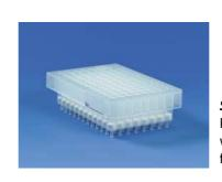
**Strep-Well HT** (25 or 50) Purification Plates with immobilized *Strep-*Tactin for high-throughput protein purification.
