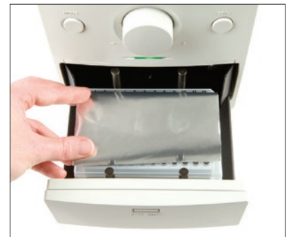
2. Place sealing film on plate.
