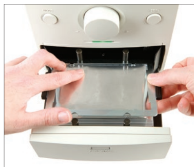
3. Place seal frame on sealing film.
