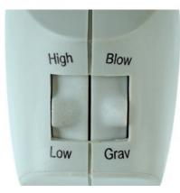
Aspiration speed can be set to HIGH or LOW to adjust for the volume of the pipet and viscosity of the liquid.
