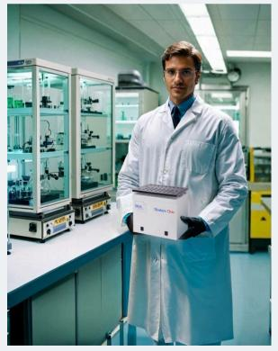
The Station One thaws frozen samples and reagents in a fraction of the time using only ambient air. Dual fans intake ambient air and channel it upward through a perforated thawing tray where it circulates over and around samples. This simple action decreases sample and reagent thawing times by up to 80% without any application of heat.
