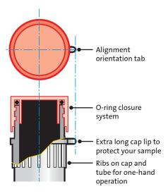
Axygen® microcentrifuge tubes are produced from virgin polypropylene that meets USP Class VI requirements.
