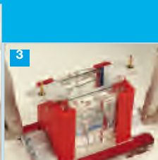
Transfer to casting base and tighten cams
