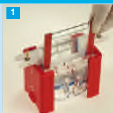
Insert glass plates and tighten screws
