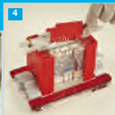
Insert gel solution and comb and allow to polymerise
