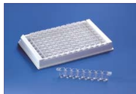
Microplate consisting of twelve 8-well strips coated with StrepMAB-Immo (see above) or Strep-Tactin ® (see below).
