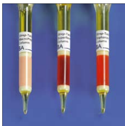
Strep-Tactin® columns regenerated with HABA (see also Strep-tag® purification cycle on page 3): Strep-Tactin® MacroPrep®, Superflow® and Sepharose® (left to right). Since MacroPrep® is not as transparent as Sepharose® or Superflow®, the color shift to red is less visible.
