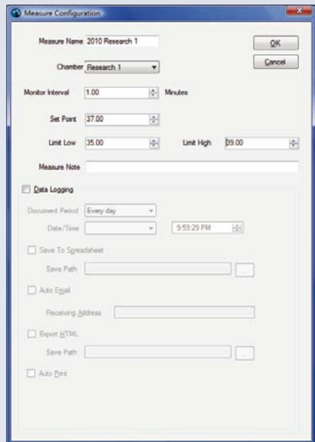
Datalogging (measurement) configuration window allow the user to easily set up the measurement interval, temperature set point, low temperature alarm point and high temperature alarm point of a chamber or an equipment. This window also allow the user to choose the method of when and which the data can be viewed (spreadsheet, e-mail, web page or print out).
