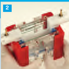
Slide doors to make efficient seal*
