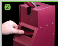
Adjust the large thumbwheel clockwise to lower the press head to the desired firm level.
