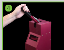
Holding the outer edge of the 'base plate', gently pull down on the handle to the bottom of its stroke and then return the handle to the top. Slide the plate tray out of the EasyPress and remove your plate.
