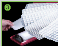
With the 'plate slide' in the out position, place the appropriate Axymat on top of the plate, align 2 - 3 corners of the Axymats and place the plate with the Axymat into the 'plate slide' and move into the press.
