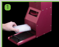
To adjust for a new plate, lower the handle and place a plate on the 'plate slide' with no Axymat.
